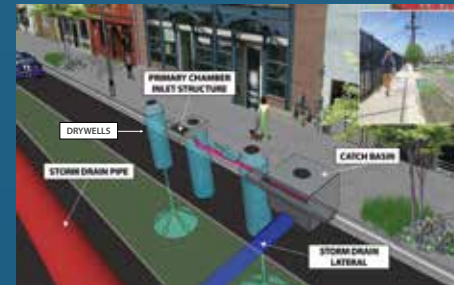
On Lankershim Boulevard in North Hollywood, we updated an existing design to provide flood control and groundwater supply benefits through the use of drywells.
