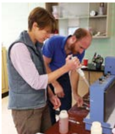
Performing jar testing for a client in Texas.
