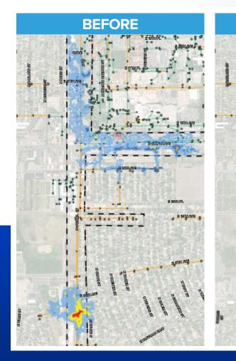
The flooding predictions for an Aurora neighborhood were modeled using InfoWorks ICM software. The results of the model for the 100-year design storm event are depicted in the above graphics, and highlight the reduction in flooding predictions once the proposed changes are completed.
